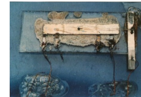
First silicon transistor, Patented 1954
